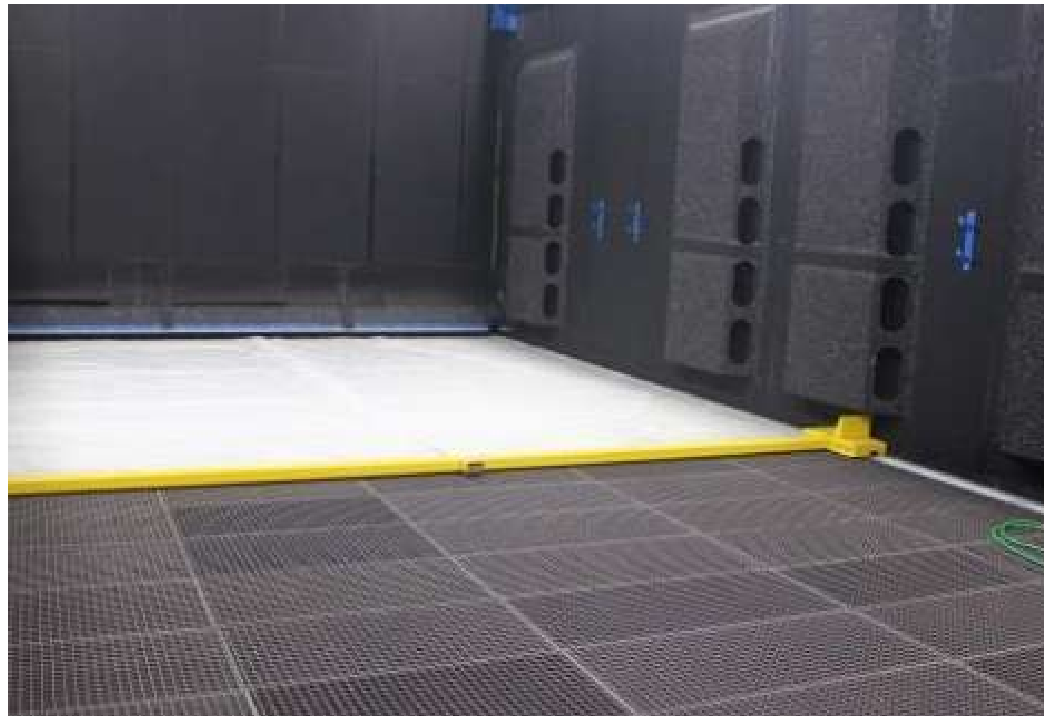
Rolling and unrolling device for the film to cover the gratings
