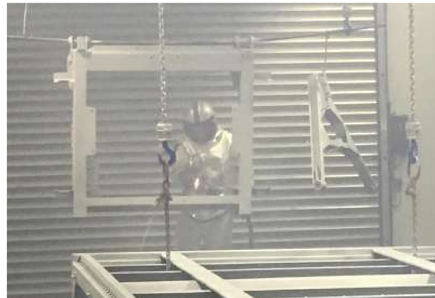
Gun metallising booth with chain hoists for suspending the parts to be treated
