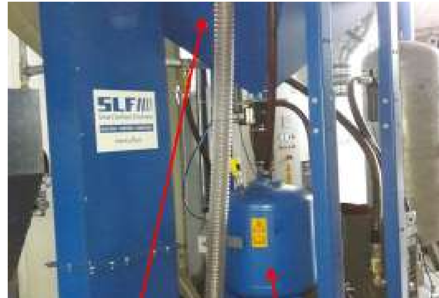
Media silo and pressure blast pot
