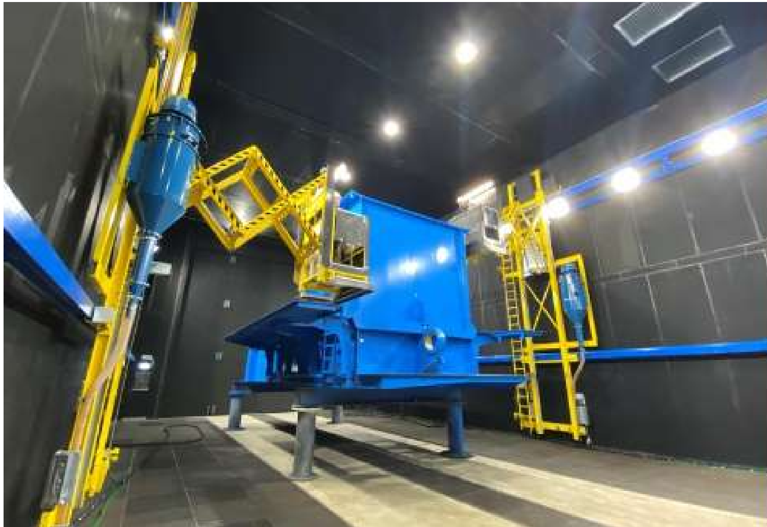
Sandblasting room with two horizontal scissor lifts guided by the side walls
