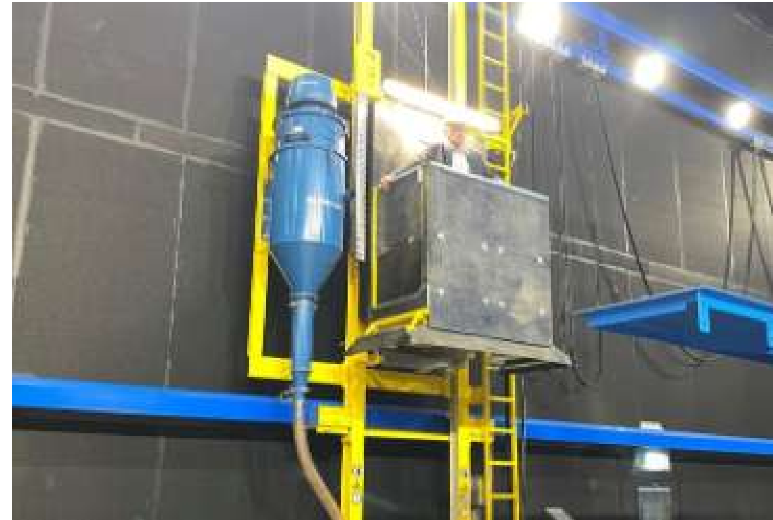
Sandblasting room with two horizontal scissor lifts guided by the side walls
