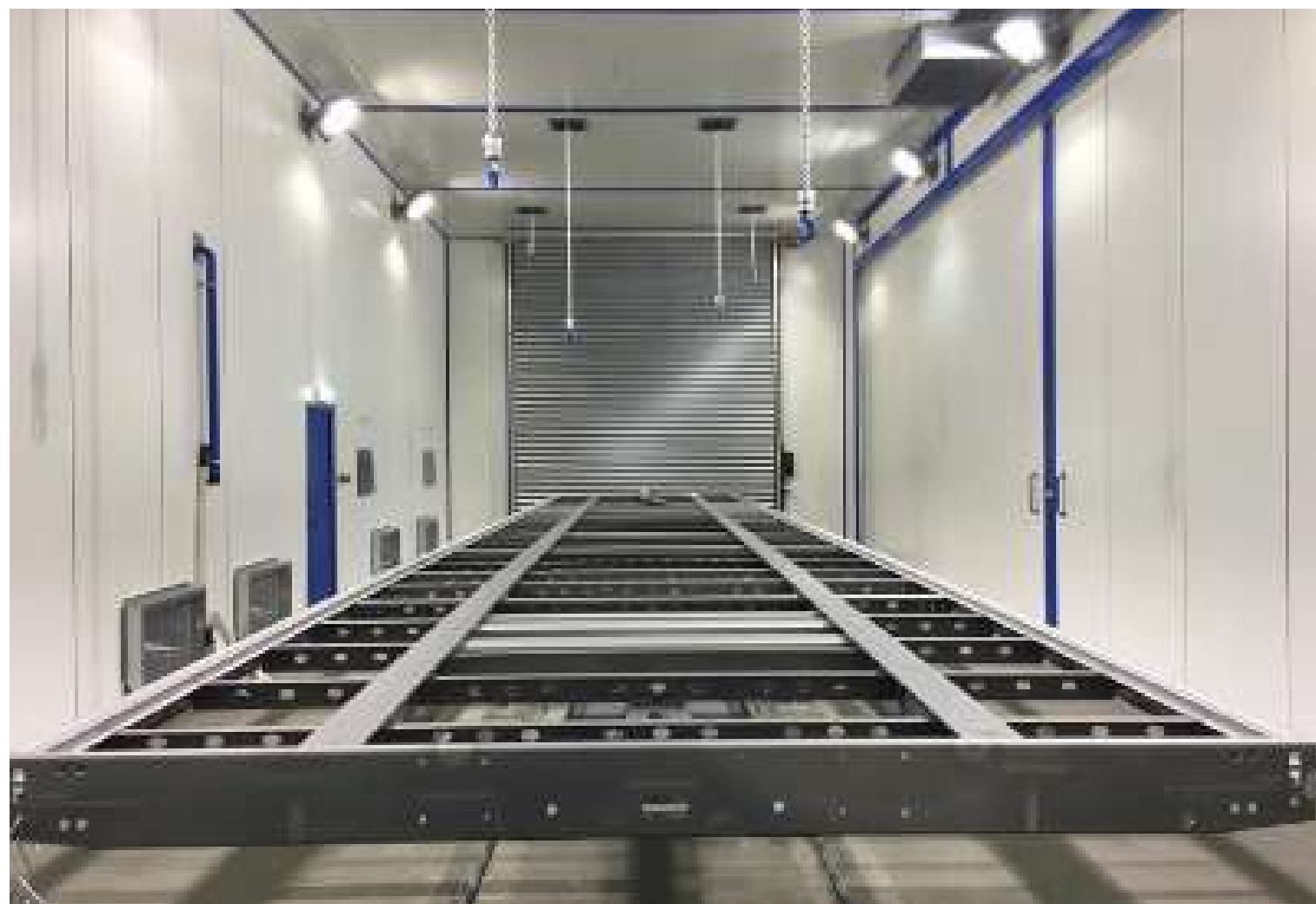
Gun metallising booth with chain hoists for suspending the parts to be treated
