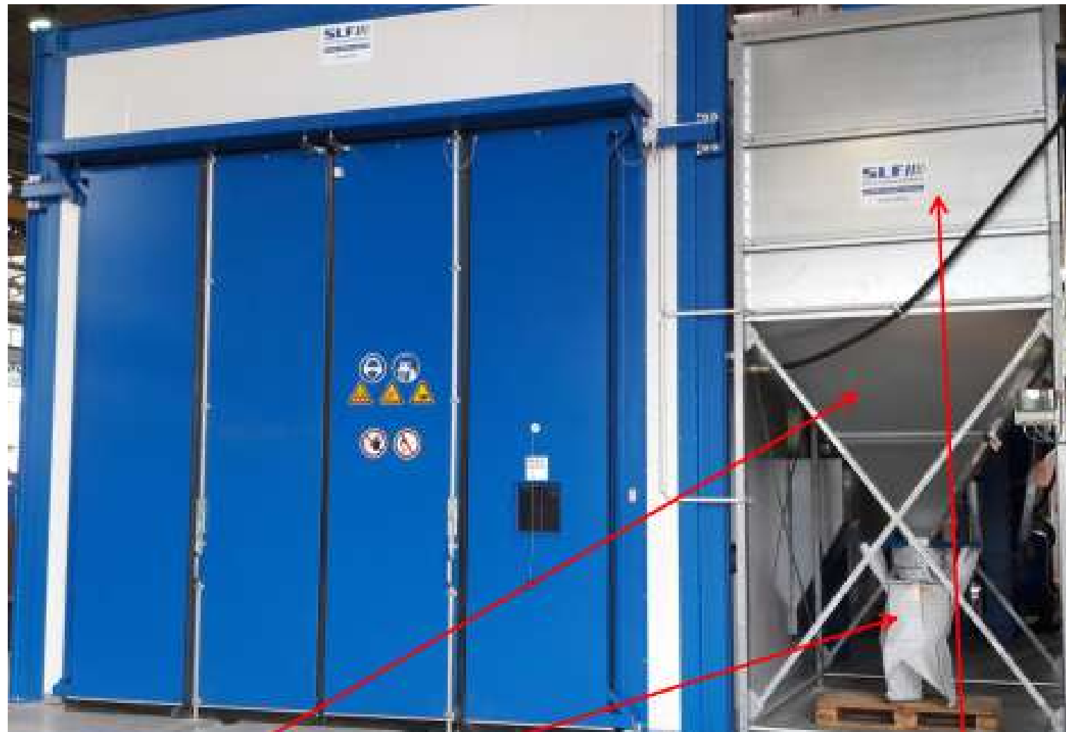
Dust collecting hopper with Big Bag to be manually emptied underneath the filter unit
